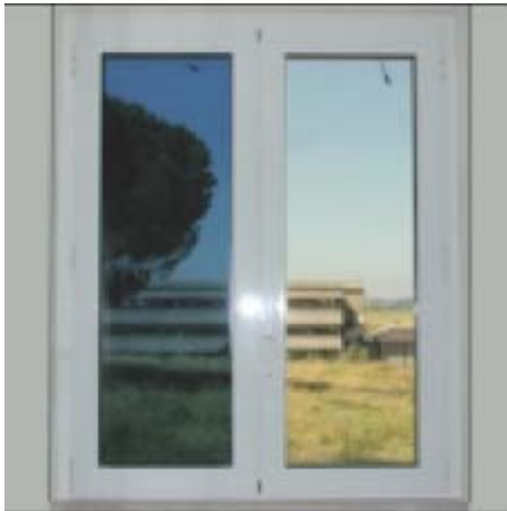
EC test window at ENEA, Italy (SWIFT project)
